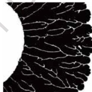
1nm CoFeB 薄膜磁畴观测
